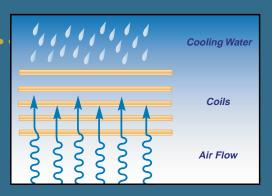
erected industrial process, refrigeration and air conditioning systems, evaporative condensers are widely used for condensing refrigerated vapor in mechanical refrigeration systems. The inherent efficiency of evaporative condensing provides lower condensing temperatures (95°) compared to other condensing methods, i.e. air cooled (115°F to 120°F) or water cooled (105°). This results in significantly reduced kW per ton (.70 system kW per ton and 17+ system EER).
